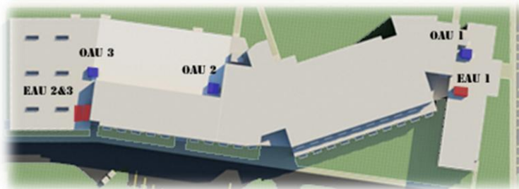
Figure 9: Air handler Layout on Second Floor Roof
